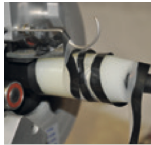
smooth and flat transition for mounting joints and terminations
