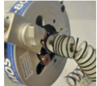
tapering the insulation
