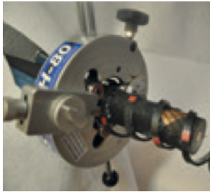
stripping of the sheath, incl. AL and Cu foil
